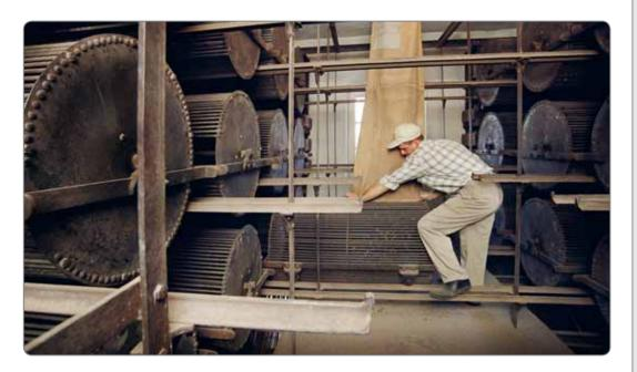
process of warming and shaking the cones to cheat out the seeds. When the cones are brought here, the bags are attached to a chain and pulled up to the second floor though the hatch by rotating the wheel. Then they are attached to linen ropes and lowered again to the first floor in cylinders resem-
